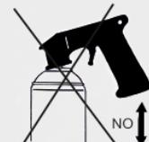
Slide handle STRAIGHT forward on can until bracket engages noticeably
